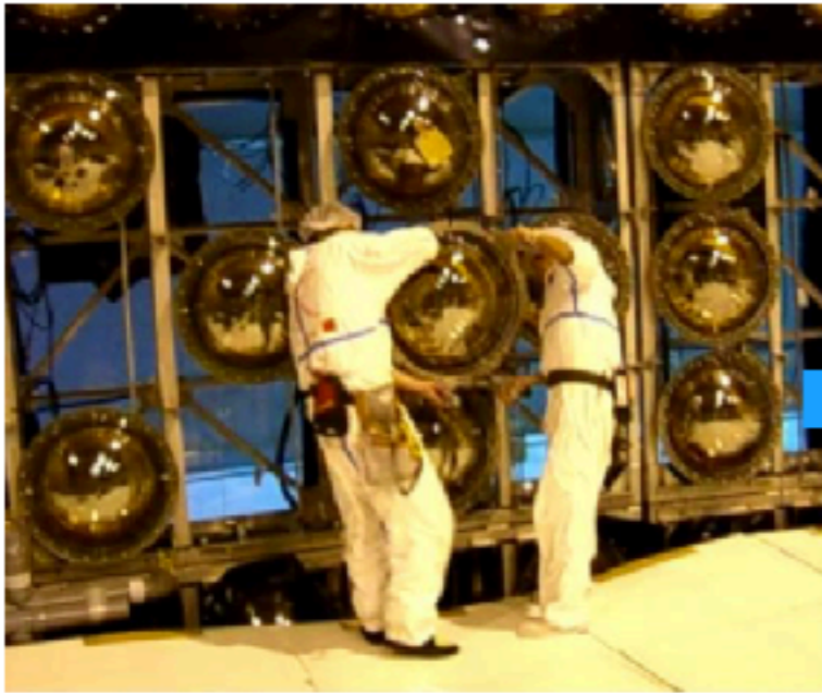
PMT / electronics installation
