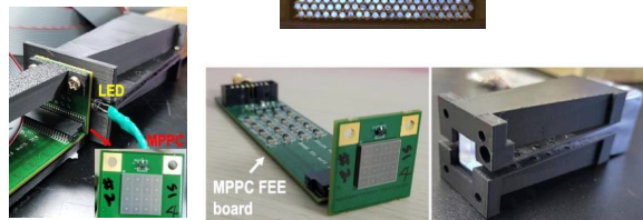
6) Connect with PMT or Light Guide + SiPM
