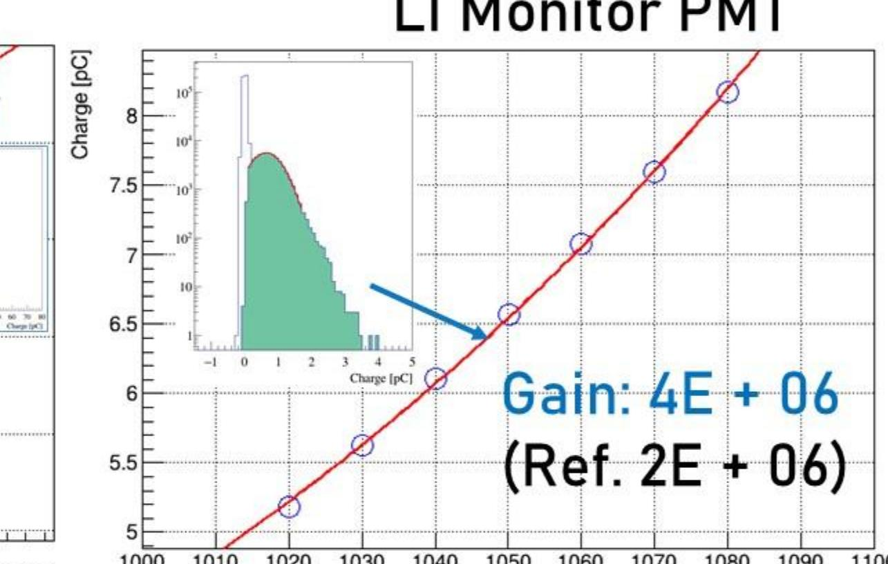
[LI Monitor PMT Gain curve]
